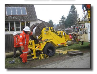
Line Surge and Galloping are eliminated by this unique hydraulic tensioning reel carrier. The system is self contained and provides smooth accurate control of the conductor tension. Ideal for use where fine control of the conductor is required or where shock loads must be avoided during fibre optic cable or special installation. An excellent Tensioner for use with a Timberland Poleboss<sup>TM</sup>.
